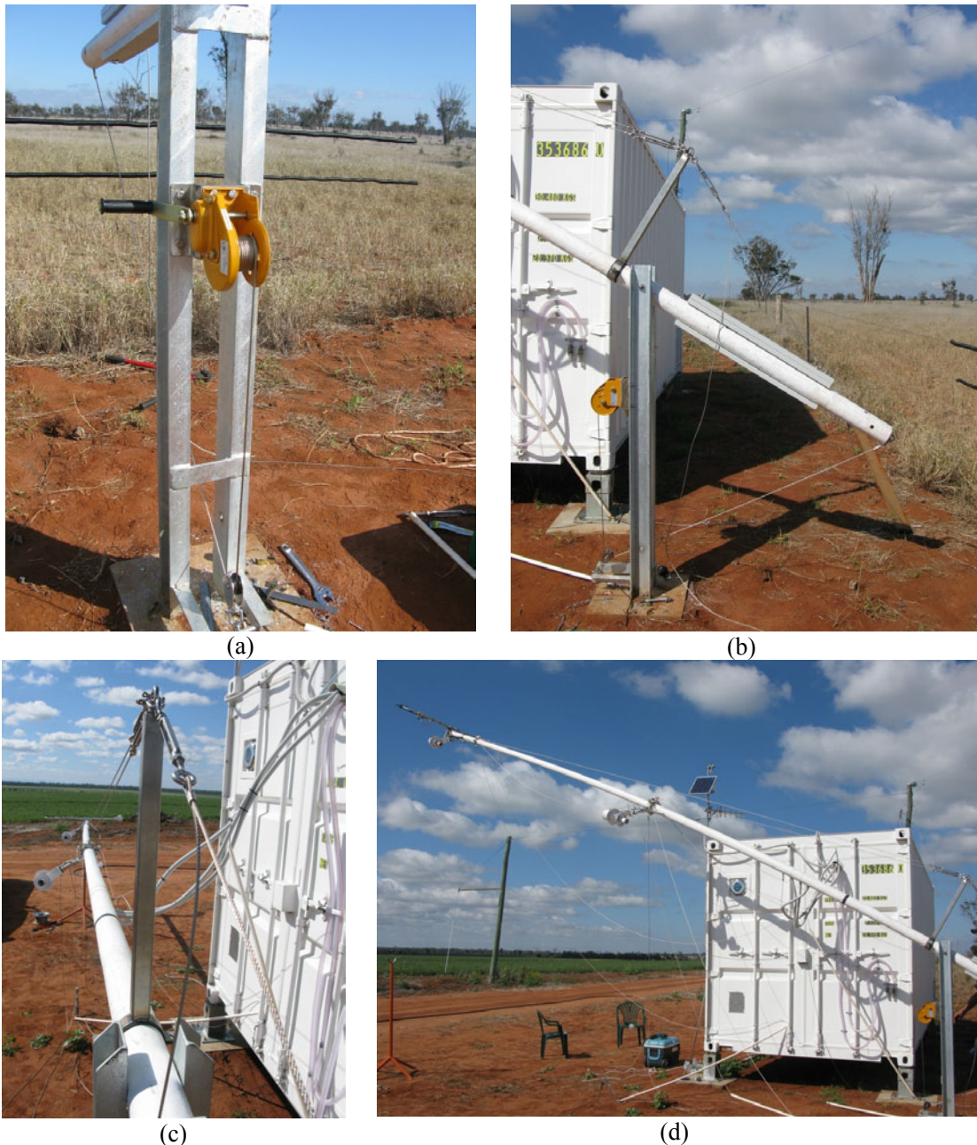
Figure 29: (a) Addition of winch to replace pulley block and cleat system for raising and lowering the mast; (b) additional counterweights bolted to end of mast to make lowering and raising the mast easier; (c) addition of stabilising bar and strength; (d) raising the mast using the winch
