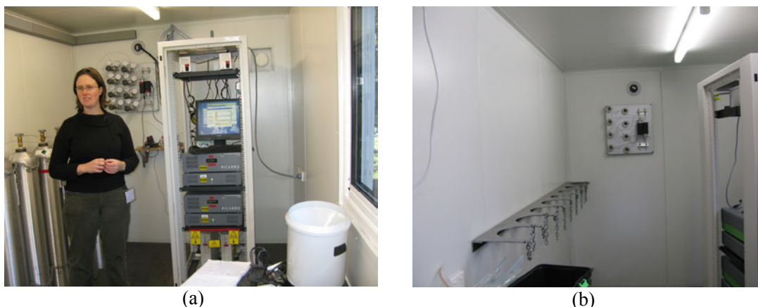
Figure 9: (a) Instrument rack to hold Picarros and UPSs; (b) Gas cylinder rack and gas regulator rack
