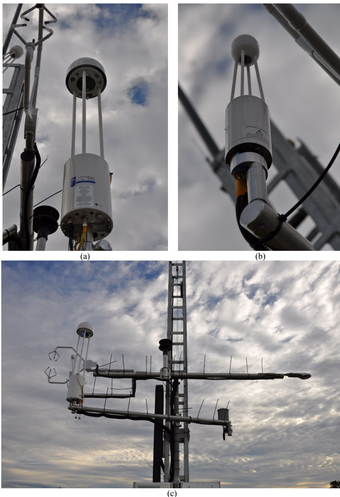
Figure 6: (a) Open path CH 4 sensor; (b) Open path CO 2 sensor; (c) Sonic anemometer (far left), CO 2 sensor, CH 4 sensor, radiometer (far right), temperature and humidity in radiation shields
