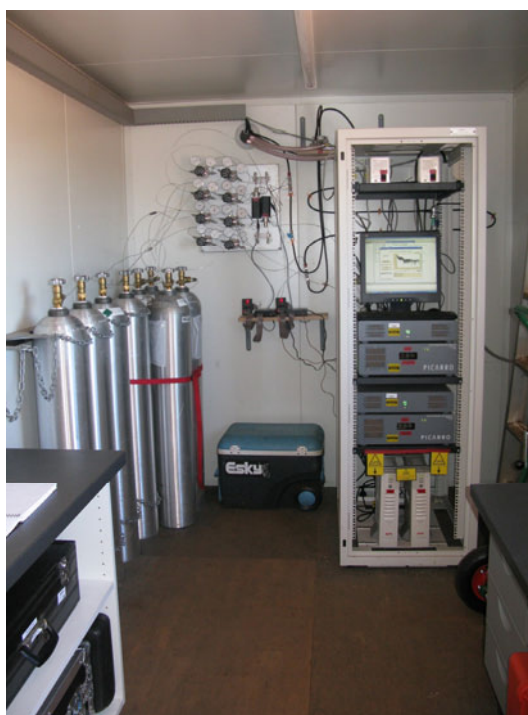
Figure 2: High precision greenhouse gas monitoring instruments (Picarro CFADS63 and CBDS36), blowers, valves, reference tanks and the original uninterrupted power supply (UPS) units installed in container at Arcturus
