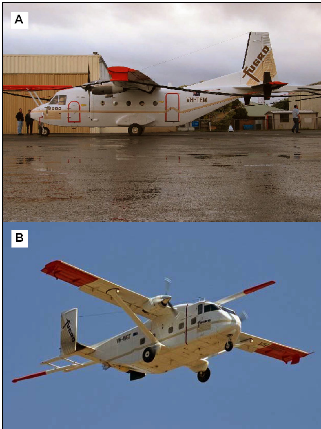
Figure 38: The two aircraft used for the TEMPEST survey. A: modified CASA 212-200 Aviocar registration VH-TEM. B: modified Shorts SC-7 Skyvan registration VH-WGT.
