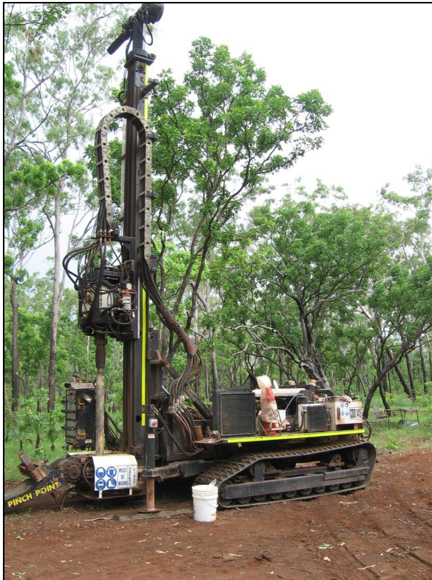
Figure 50: Boart-Longyear Delta base 320 sonic drill rig on site at RN37150.
