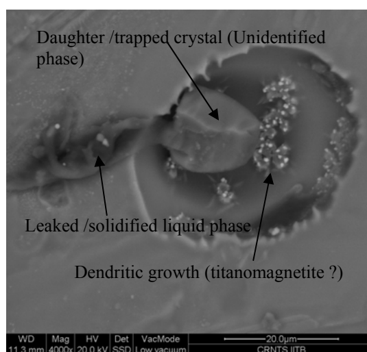
Figure.2 Backscattered ESEM photograph of melt inclusion (break open cavity)
