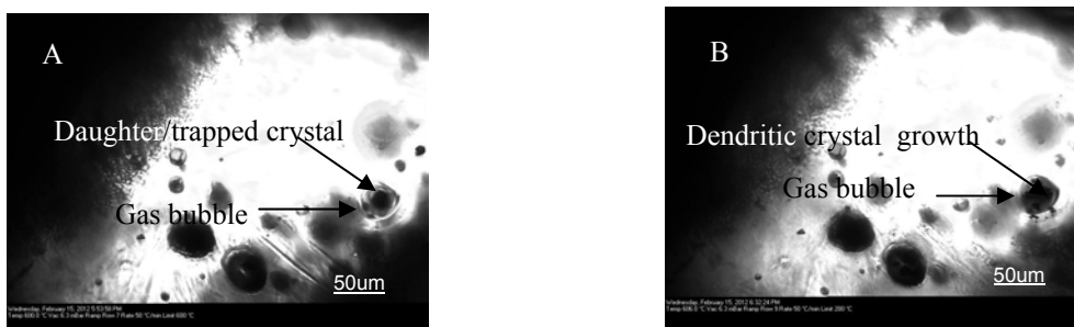
Figure.1 Microphotograph of Biphasic melt inclusion (Gas bubble + Solid) during heating (A) and cooling (B) experiment.
