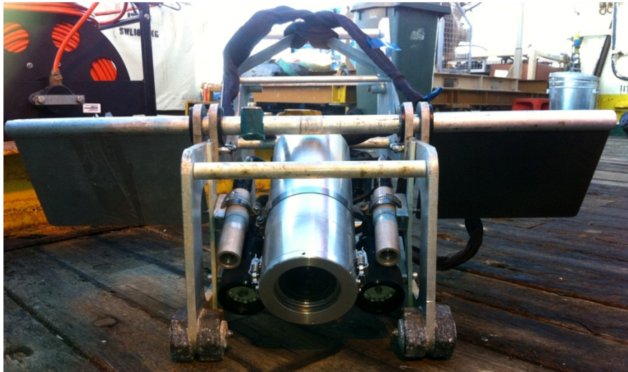
Figure 2.6: Towed Video System. Raytech towed-camera showing the forward facing camera, light mountings and two lasers.
