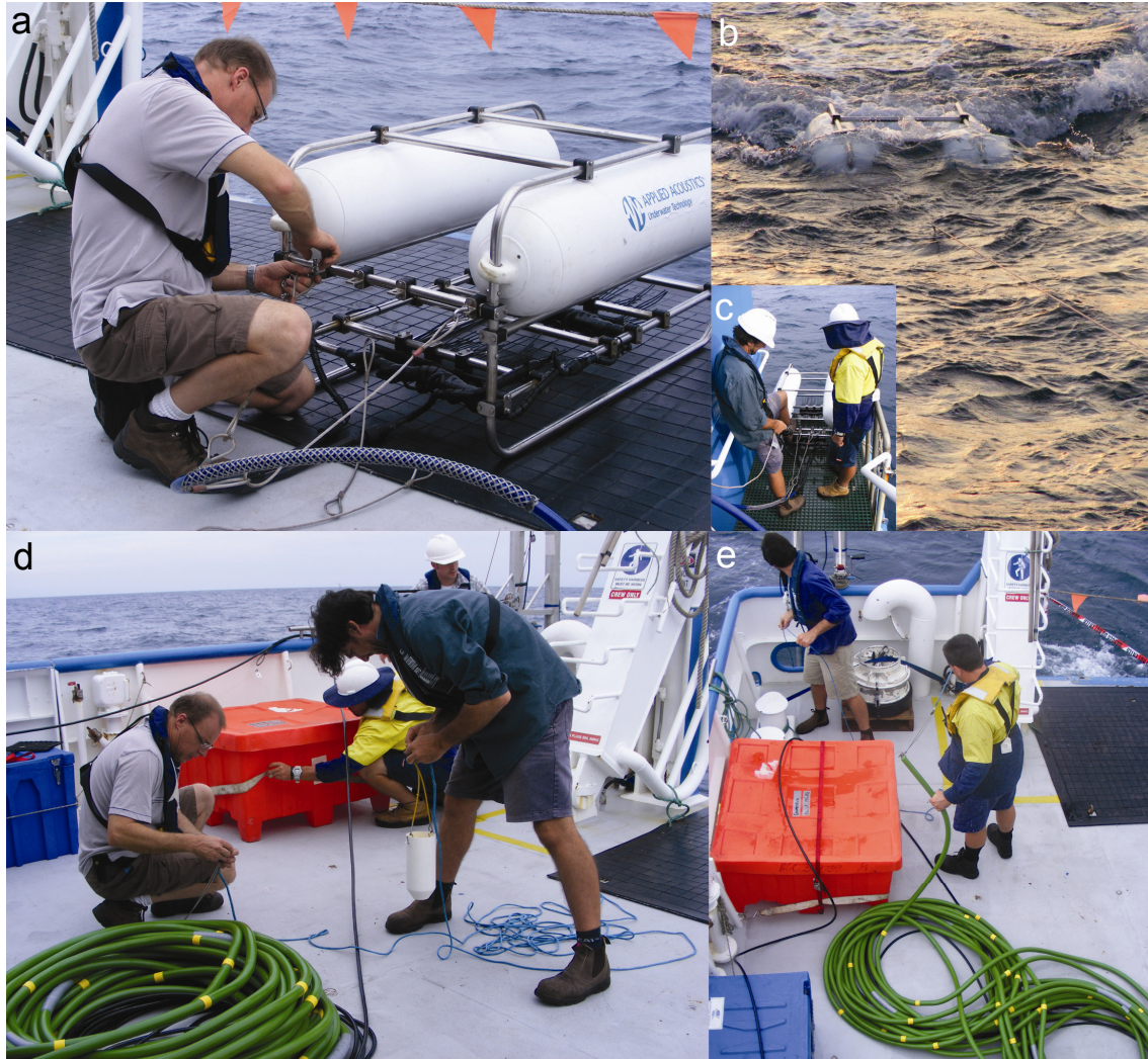
Figure 2.1: (a-c) Preparation and deployment of the Applied Acoustics Squid 2000 “Sparker” sub-bottom profiler and (d-e) 24 channel Geometrics Geoeel.
