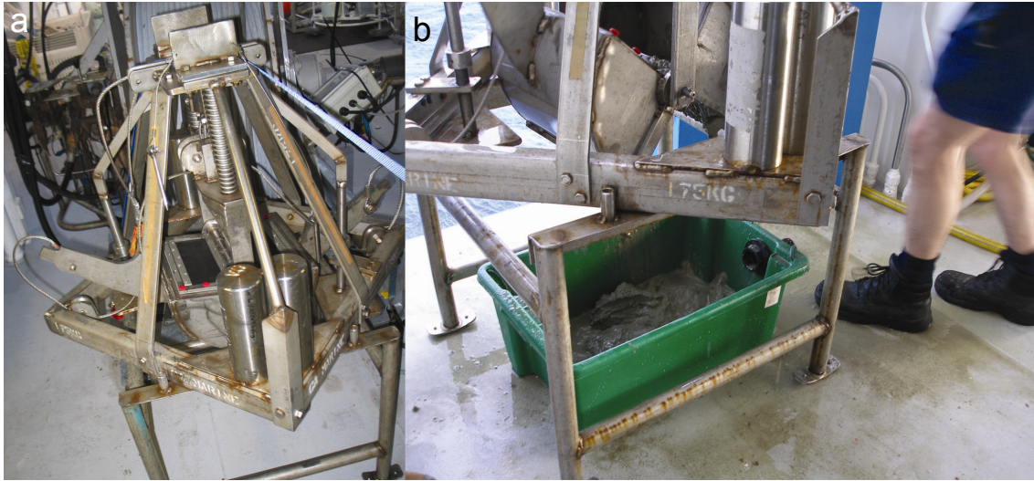
Figure 2.5: (a) Smith McIntyre grab used to collect seabed samples (b) for sediment grain-size analyses, geochemistry and infauna.
