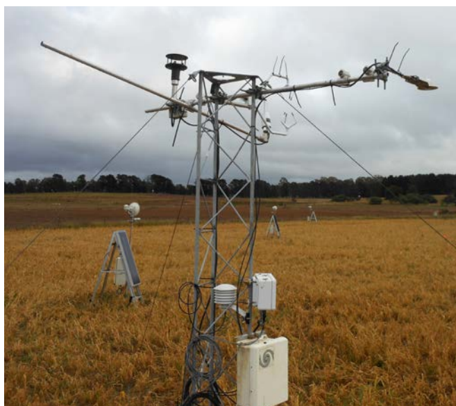
Figure 1: Wireless network of solar powered CO 2 sensors and eddy covariance tower at the GA-CO2CRC Ginninderra greenhouse gas controlled release facility, Canberra.
