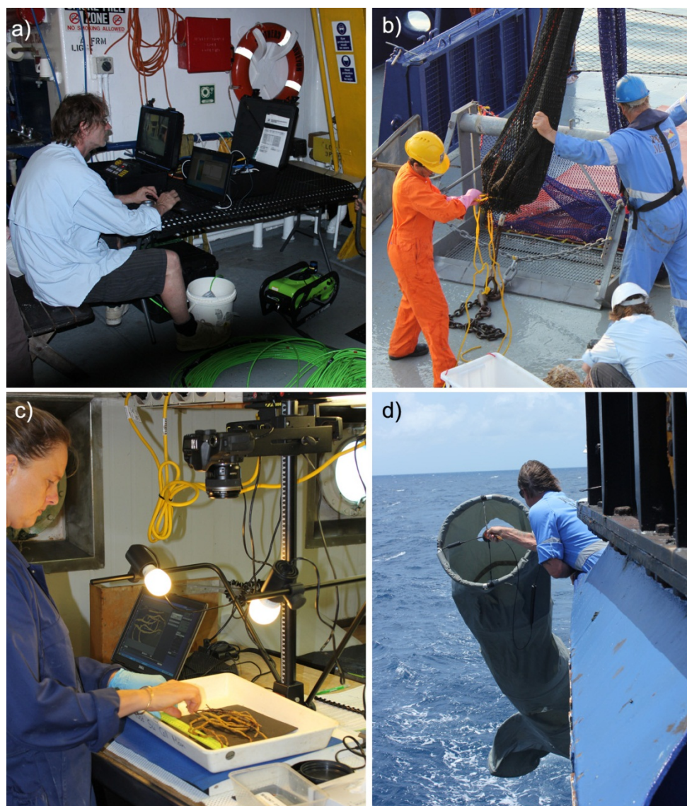
Figure 2.1: Equipment and methods used to collect specimens and data. a) Seabotix ROV (bright green and black) with live video feed to surface, b) Australian Institute of Marine Science benthic sled, c) Processing sled specimens in the laboratory, d) NOAA ocean drifter.
