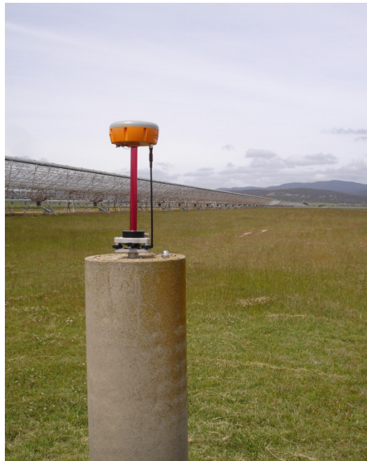
Figure 2: GNSS campaign survey set-up at the West Pillar (CAPW)
