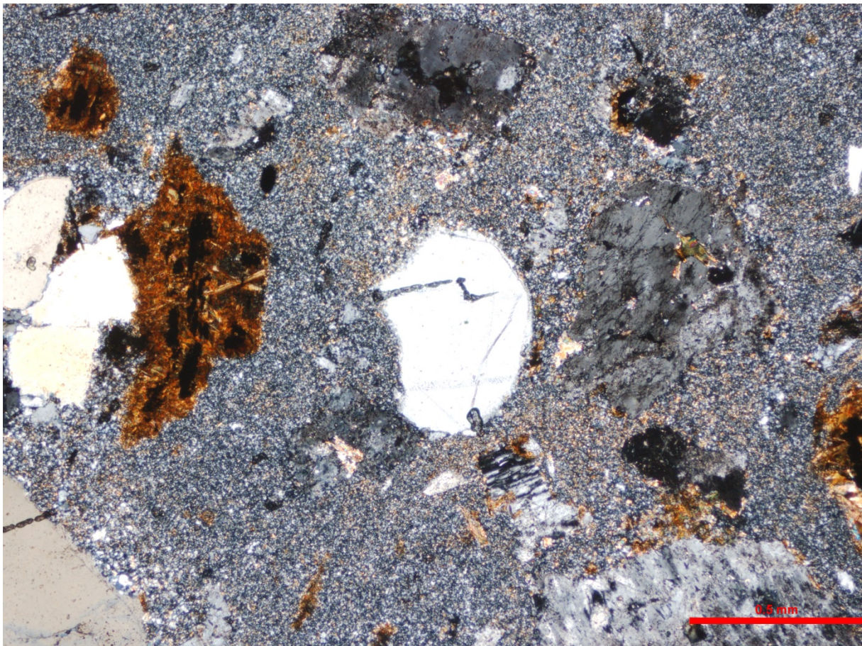
Figure 5.2 Representative photomicrograph of the Wandsworth Volcanic Group 'Kurrajong Park volcanics', at Honeysuckle Hills (GSNSW: BB-10-WVG-08, GA: 2120077) in cross-polarised light. Dacitic ignimbrite with phenocrysts of albitised plagioclase, quartz and ferromagnesian minerals/biotite replaced by fine decussate biotite and a finely microcrystalline quartzo-feldspathic matrix. Scale bar is 0.5 mm. Image supplied by Geological Survey of NSW.
