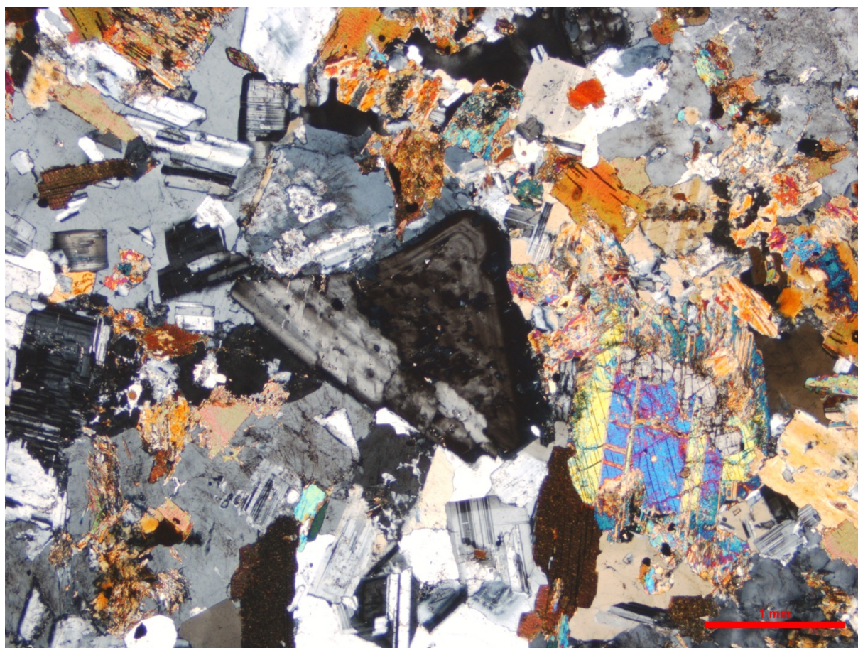
Figure 7.1 Representative photomicrograph of the Khatoun Tonalite (GSNSW: PB-12-URA-01, GA: 2129544) in cross-polarised light. Inequigranular tonalite with relatively well-formed plagioclase crystals (e.g. centre and below), interstitial and micropoikilitic (top left) quartz and alkali feldspar (top right and lower left). Clinopyroxene partly mantled by fibrous amphibole (right of centre) and small hornblende grains on right and upper margins of the photo, along with stumpy biotite laths (mainly orange in this view). Scale bar is 1 mm. Image supplied by Geological Survey of NSW.
