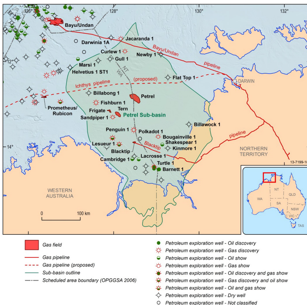
Figure 2.5 Petrel Sub-basin gas fields and pipeline infrastructure including the hydrocarbon shows of the petroleum exploration wells. Key wells for petroleum exploration in the Petrel Sub-basin labelled.
