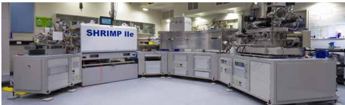
The Sensitive High-Resolution Ion Microprobe (SHRIMP) for precise age determination of Australia's rocks.
