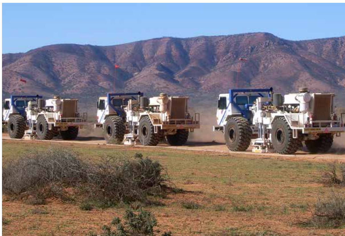
Vibroseis trucks acquiring deep seismic reflection data in the Flinders Ranges, South Australia.
