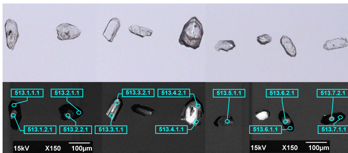
Figure 3.2 Representative zircons of the unnamed granite at R7 Prospect (GSNSW: PB-11-NYM-16, GA: 2128513). Transmitted light images are shown in the upper half and cathodoluminescence images in the lower half. SHRIMP analysis sites are labelled with sample (prefix 2128- not annotated), grain, spot and replicate number. Scale bar is 100 \mu\text{m} .
