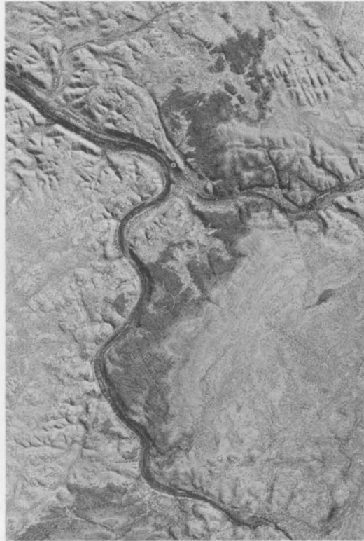
Plate 13. Distinctive photo-pattern of the Supplejack Dolomite Member of the Skull Creek Formation. The very dark tone results from the low reflectivity of the bare irregular surfaces of massive dark grey dolomite. Dolomite and siltstone above and below the member form light-coloured soil and support grasses which increase reflectivity. Aerial photographs at 1:85 000 scale. The area shown is 10 km northwest of Bullita homestead; the East Baines River traverses the centre of the photograph. (Waterloo RC9, Run 1, Photos 82, 84)
