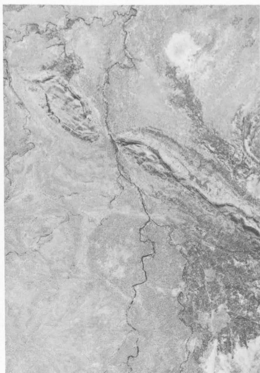
Plate 27. Northwesterly-trending closed anticlines developed in the Skull Creek Formation in the southwestern Delamere Sheet area. The anticlines are faulted, and displacement of the Supplejack Dolomite Member (dark-toned bed outlining the structures) demonstrates left-lateral movement of about 300 m with little or no vertical displacement. (Delamere RC9, Run 8, Photos 18, 20)
