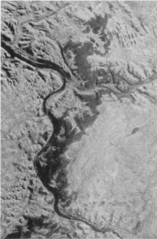
Plate 13. Distinctive photo-pattern of the Supplejack Dolomite Member of the Skull Creek Formation. The very dark tone results from the low reflectivity of the bare irregular surfaces of massive dark grey dolomite. Dolomite and siltstone above and below the member form light-coloured soil and support grasses which increase reflectivity. Aerial photographs at 1:85 000 scale. The area shown is 10 km northwest of Bullita homestead; the East Baines River traverses the centre of the photograph. (Waterloo RC9, Run 1, Photos 82, 84)
