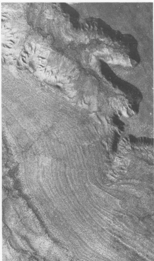
Plate 14. Distinctive photopattern and terraced topography of the Skull Creek Formation. The broad dark band in the lower left corner is the Supplejack Dolomite Member, which is overlain by interbedded dolomite and dolomitic siltstone. These produce the banded photopattern in the centre of the photograph. The terraces on the right are developed at the Skull Creek/Bynoe Formation contact, a gradational boundary in which the siltstone content increases upwards. The mesa consists of flat-lying Jasper Gorge Sandstone. About 20 km south-southwest of Bullita homestead. (Waterloo K17, Run 4, Photos 05, 06)
