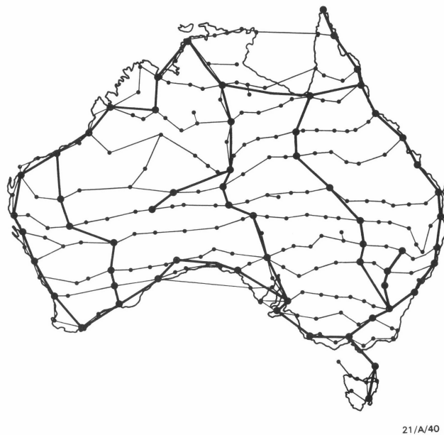
Figure 2. Australian gravity base-station network in 1980.
