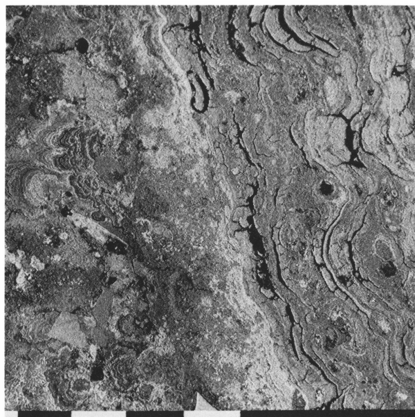
Figure 4. Scanning electron microscope (SEM) micrograph of polished section of Dampier Ridge ferromanganese oxides (Station 57), showing complex layering of ferruginous vernadite (dark) containing thin layers of todorokite (light).
