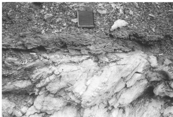
Figure 3. Road cut exposure in Esperance area, illustrating iron-cemented sediments overlying weathered steeply dipping rocks with a marked unconformity. Note the truncated quartz veins and the black maghemitic pisoliths at the surface. Notebook measures 10 x 7 cm.
