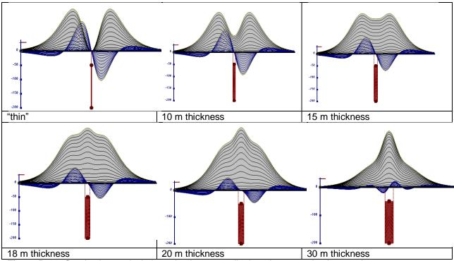
Figure D-16: Conductive vertical plate, depth 50 m, strike length 200 m, depth extends 150 m.
