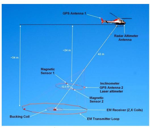
Figure 5: VTEM<sup>plus</sup> System Configuration.
