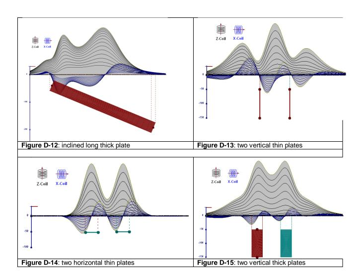
The same type of target but with different thickness, for example, creates different form of the response:
