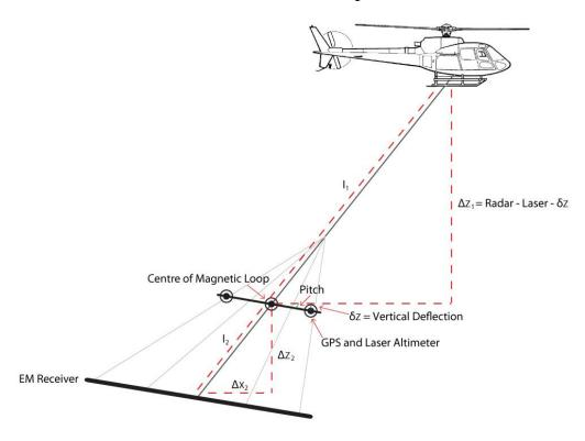
Figure 8: Calculation of EM transmitter loop height.
