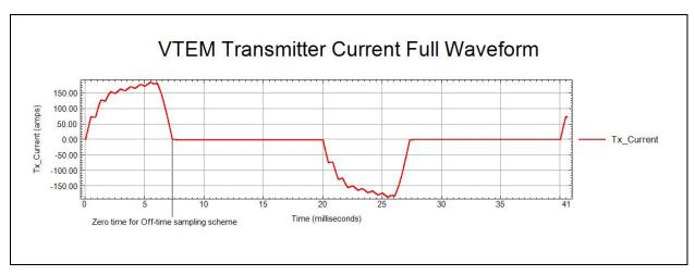
Figure 4: VTEM Transmitter Current Waveform
