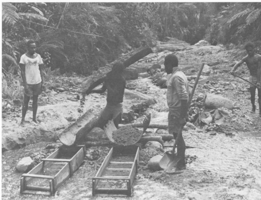
Fig. 35. Villagers groundsluicing in Namba Wan Gold Creek (at the head of Parchee Creek), East Sepik Province, in 1973. River gravels, originally mined before World War II, are being reworked for small returns. (M/1485/13)
