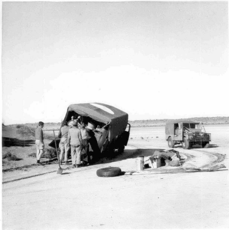
The Commer truck broke through the surface salt crust on a small lake NW of Lake Dora. It is particularly treacherous at the point of a dune (shown on the left of the photo) where seepage adds to the softness of the salt crust.
