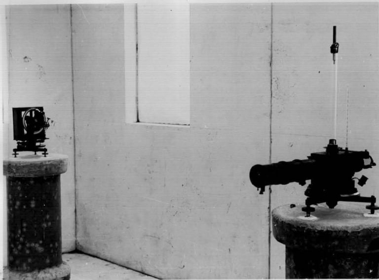
(c) Dip-circle and magnetometer on the piers in the absolute magnetic hut.
