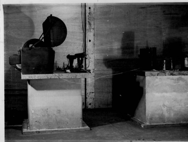
(c) Wood-Anderson type horizontal component seismographs with recording drum.
