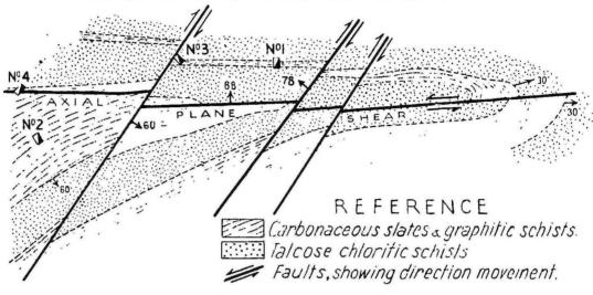
DIAGRAMMATIC TRANSVERSE SECTION showing possible recurrence of ore.
