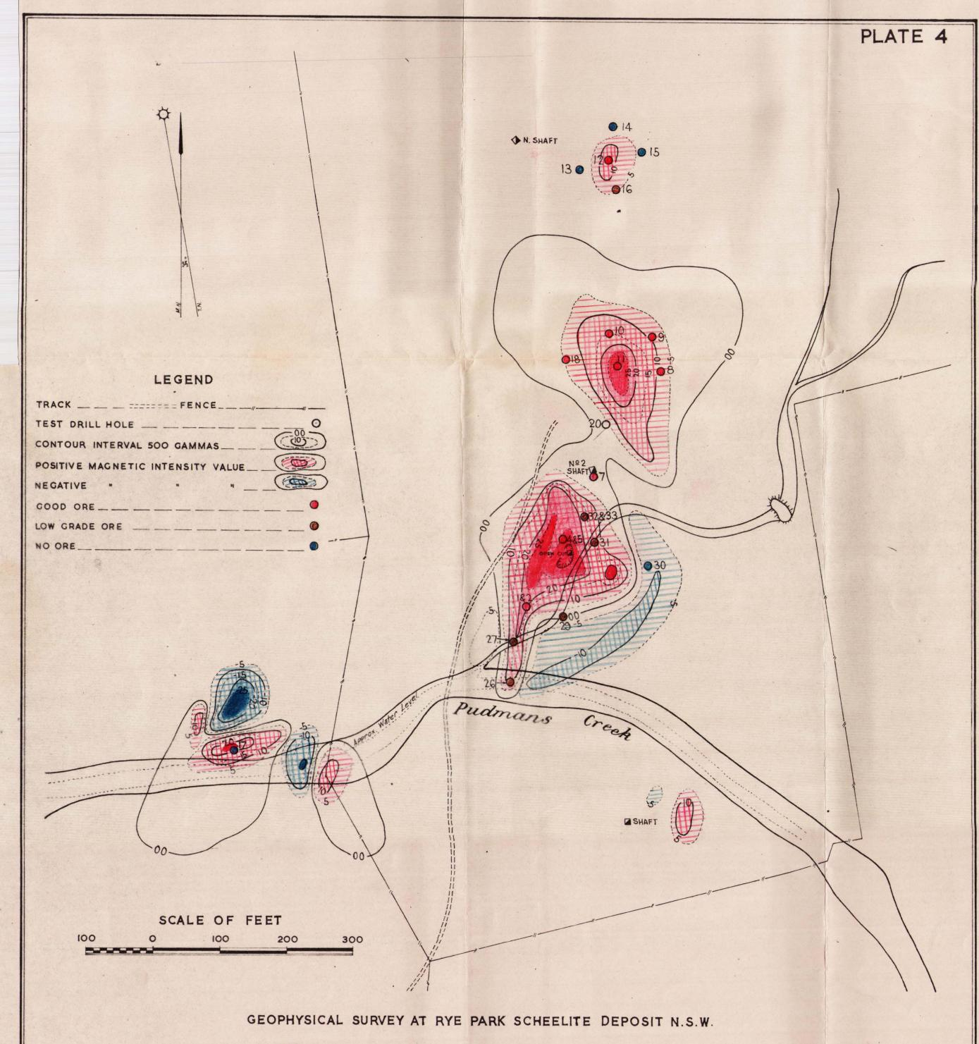
POSITION OF TEST DRILL HOLES IN RELATION TO MAGNETIC ANOMALIES
