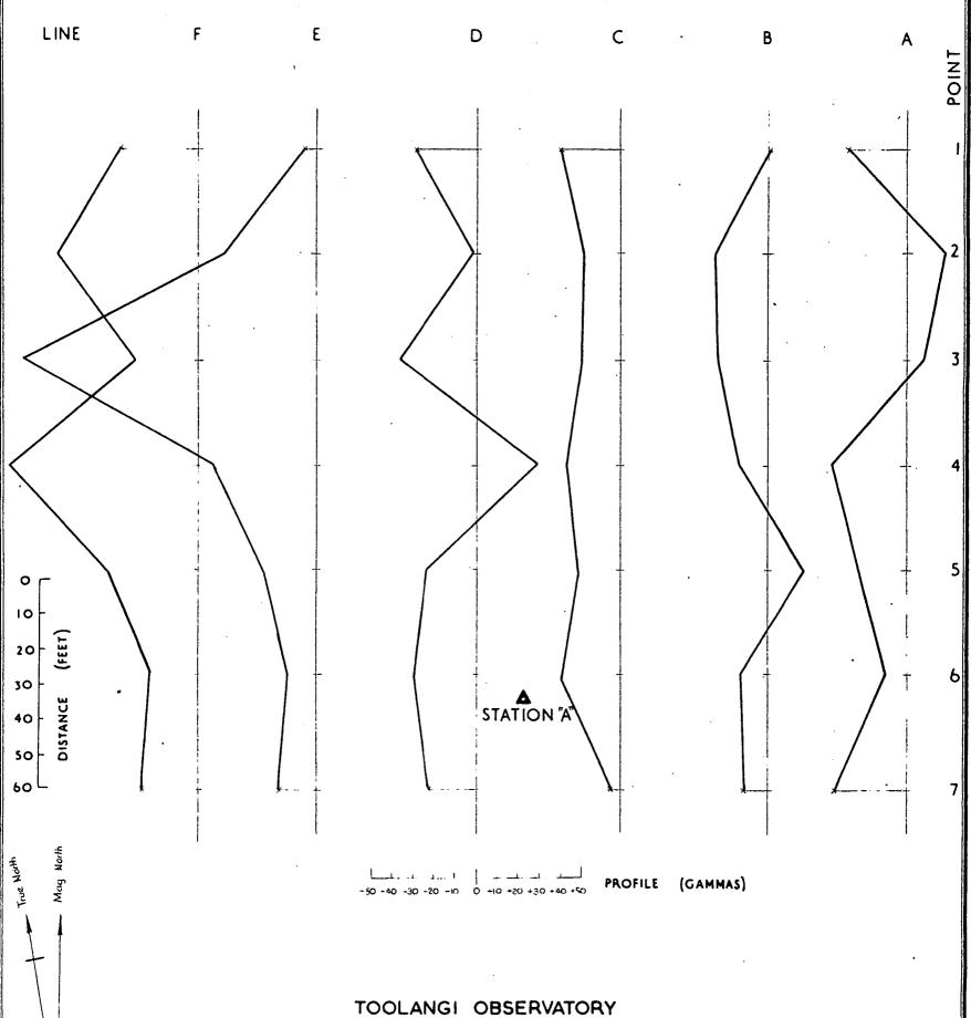
PROFILES SHOWING DEPARTURES IN VERTICAL INTENSITY FROM STATION "A"
