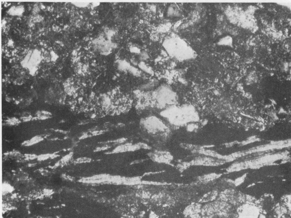
Fig. 52. Fine-grained sandstone in which sparry carbonate, probably siderite, partly replaces carbonaceous material and fills interstices between shreds. Core at 120 m, BHP 2, Blackwater. Crossed polarizers, x 160.
