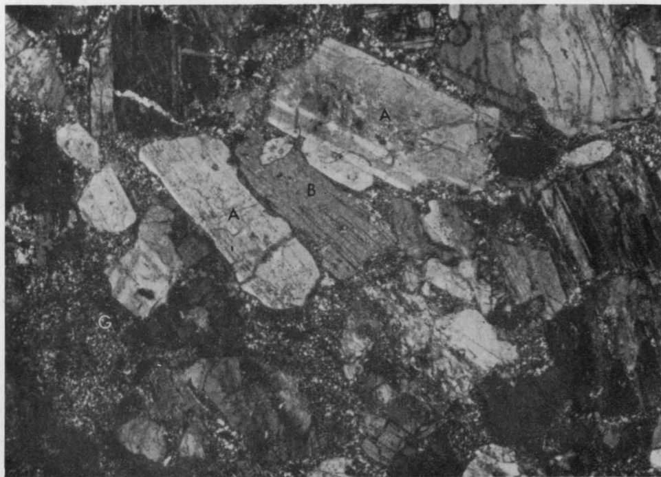
Fig. 6. Crystal tuff of the Kaloola Member of the Baralaba Coal Measures. The rock consists of crystals of andesine (A) and biotite (B) set in recrystallized glassy groundmass (G). Crossed polarizers, x 40.
