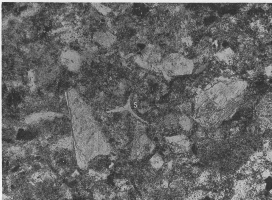
Fig. 5. A glass shard (S) in very fine-grained sandstone of the Burngrove Formation, Central area. Plane polarized light, x 160.
