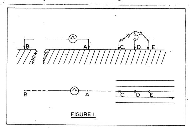
Current from a 500 c.p.s. generator is supplied to the earth through two electrodes A and B, (See fig. 1.) which are about 3,000 ft. apart. A series of parallel traverses is pegged out approximately in line with AB, and working away from the electrode A.
