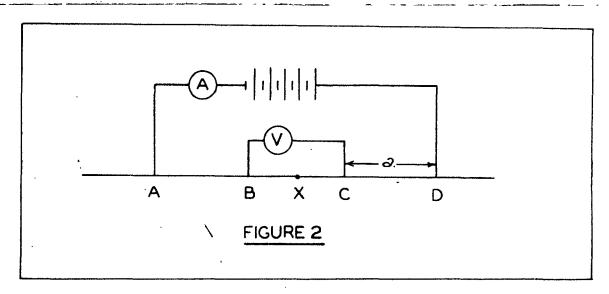
from batteries through the electrodes A and D. The resulting voltage across the inner electrodes B and C is then measured by a D.C. potentiometer. From this voltage and the current, the "apparent" resistivity of the earth, corresponding to the electrode separation 'a' can be calculated. For very small electrode separations, this is equal to the true resistivity of the surface layer; as 'a' is increased, the effect of layers at depth becomes important.
