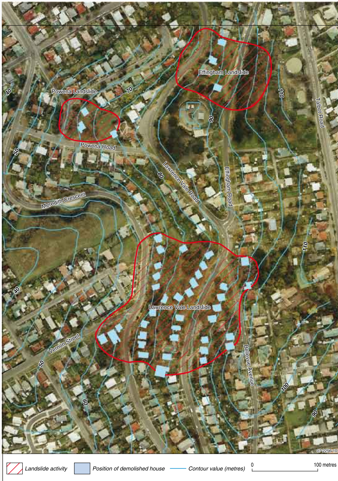
Figure 2.12: Orthophoto of Lawrence Vale, Tasmania, where over 40 houses were destroyed by landslide activity in the period from the 1950s to the 1970s
