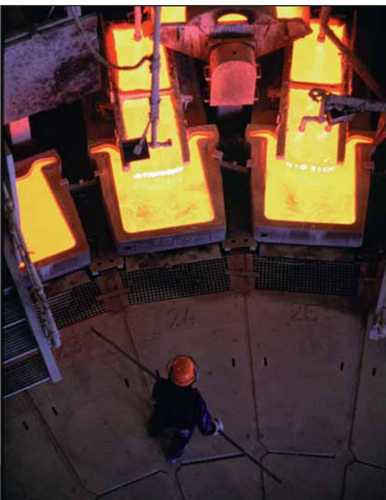
Plate 5 Copper anode casting wheel at MIM's Mount Isa smelter operation Photograph courtesy of MIM Holdings Ltd
