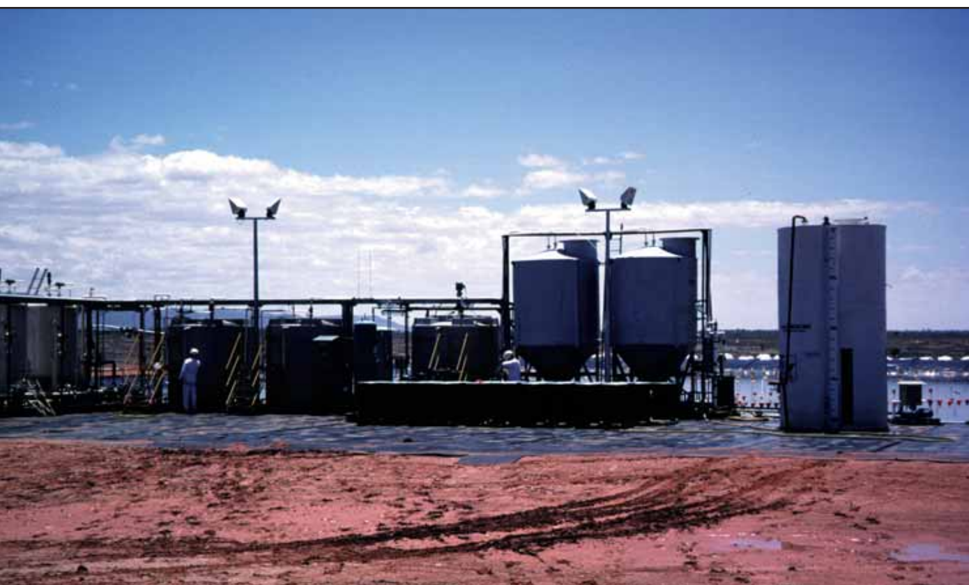
Plate 8 Ion exchange columns for in situ leach trials at the Beverley uranium project, South Australia Photograph courtesy of Aden McKay, AGSO; published with the permission of Heathgate Resources Pty Ltd
