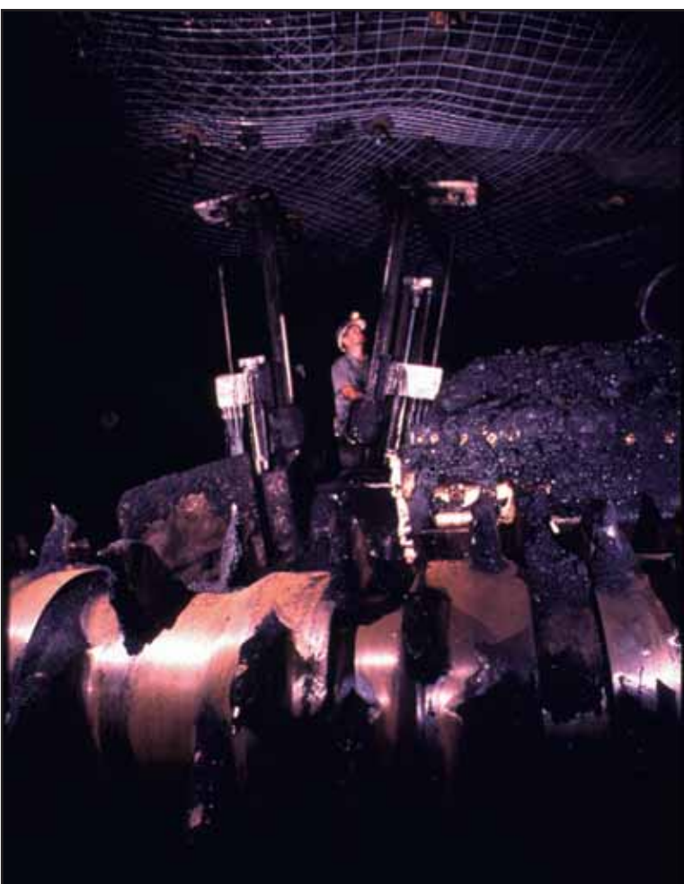
Plate 4 Roof bolting in preparation for longwall mining at Oaky Creek's second underground mine, Queensland Photograph courtesy of MIM Holdings Ltd
