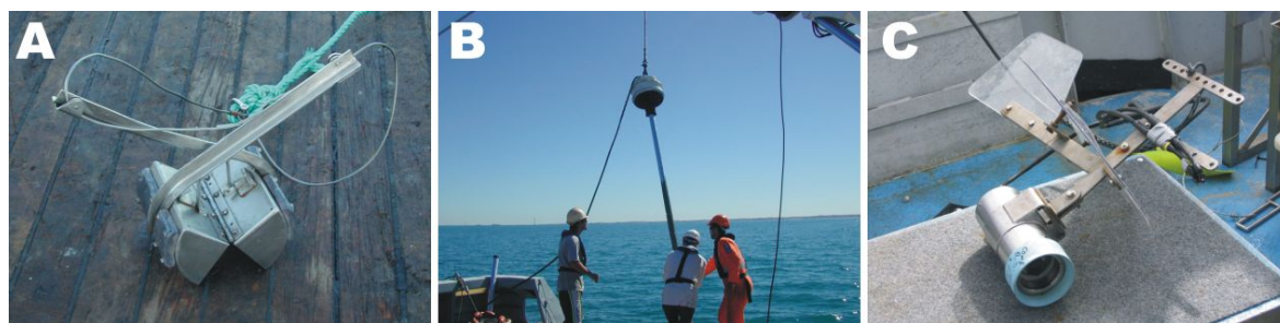
Figure 5: Sediment sampling and underwater video equipment used in this study. A) Van-veen type grab sampler; B) Submersible vibracorer; C) Towed underwater video camera used by the CWHM team from University of Western Australia.
