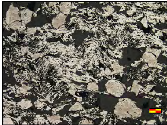
Figure 6. CAP3143 higher magnification reflected light photomicrograph showing crenulated micaceous hematite and martitised magnetite porphyroblasts. Scale-bar 100 microns.
