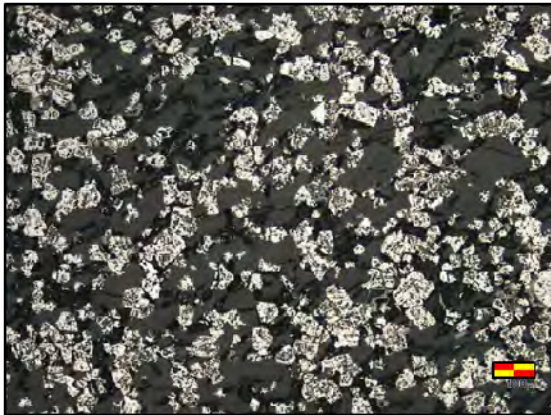
Figure 5. CAP3120 reflected light photomicrograph showing subhedral martitised magnetite and quartz-biotite matrix. Scale-bar 100 microns.
