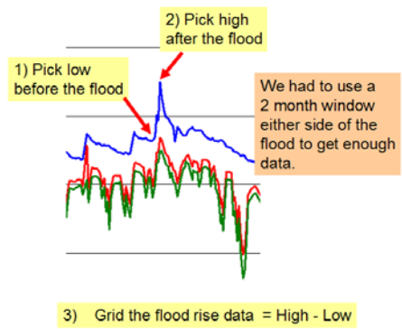
Figure 7: Borehole hydrograph flood analysis steps.
