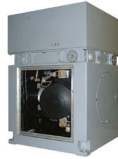
Figure 3. Photograph of the GT-1A gravimeter from the side, with cover removed showing the gyro-stabilized platform contained in a double-axis gimbal suspension.
