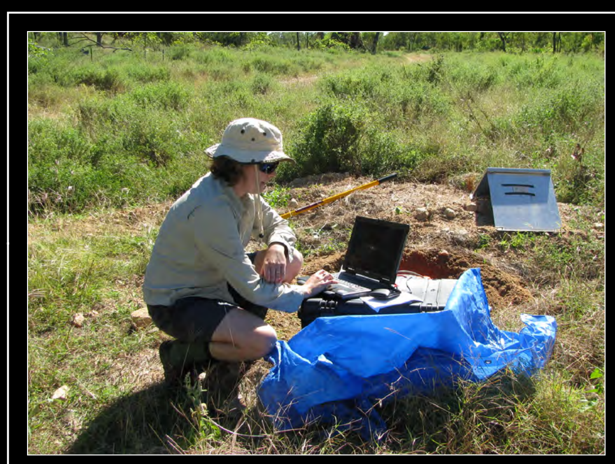
Setting up temporary seismometer for aftershock deployment after Bowen earthquake 2011.
