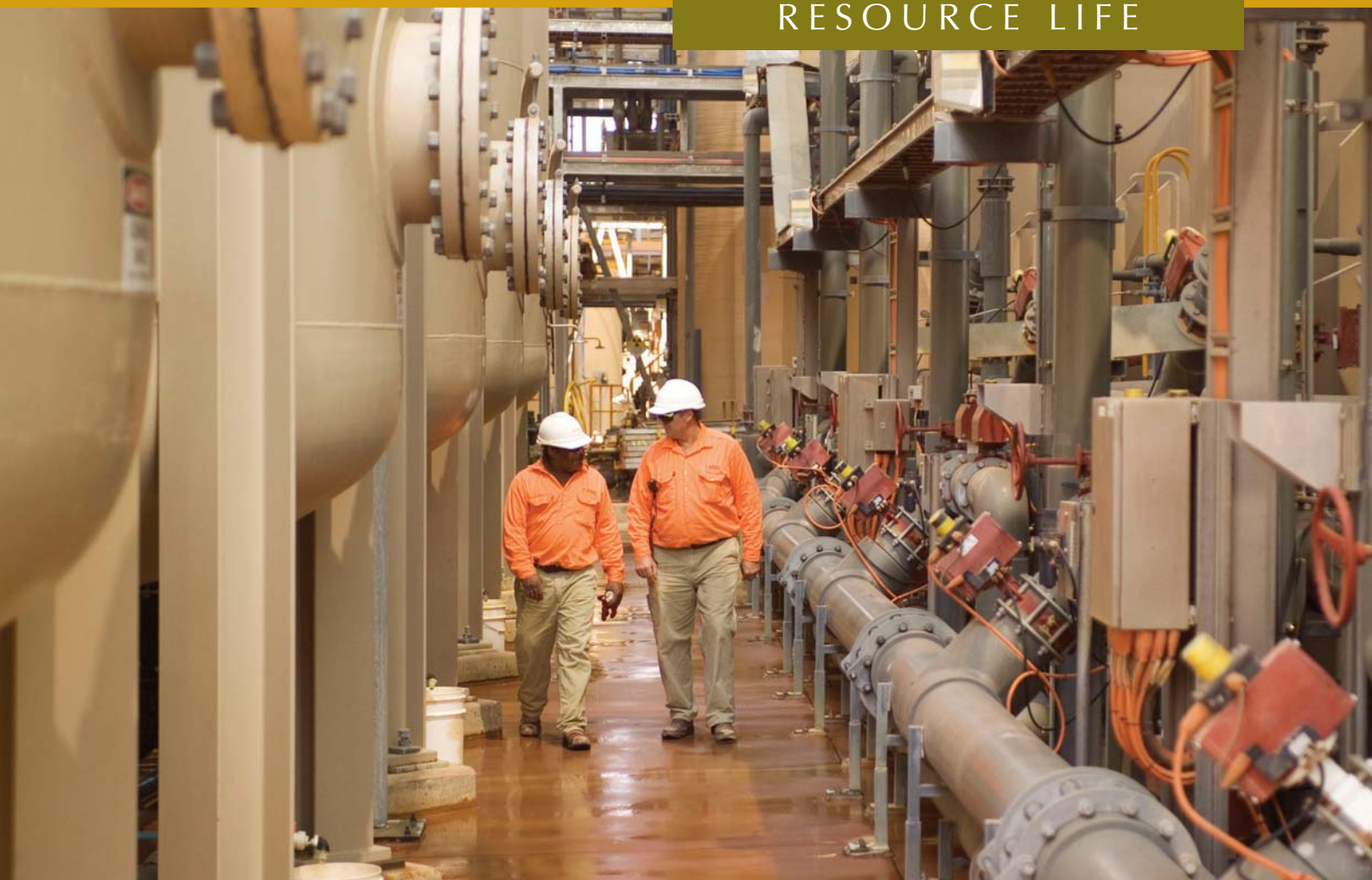
Uranium extraction plant using ion exchange technology at Beverley mine, South Australia (Heathgate Resources Pty Ltd).
