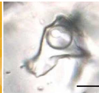
▶ Figure 4b. Photomicrographs of CO 2 -rich fluid inclusions from The Granites goldfield
