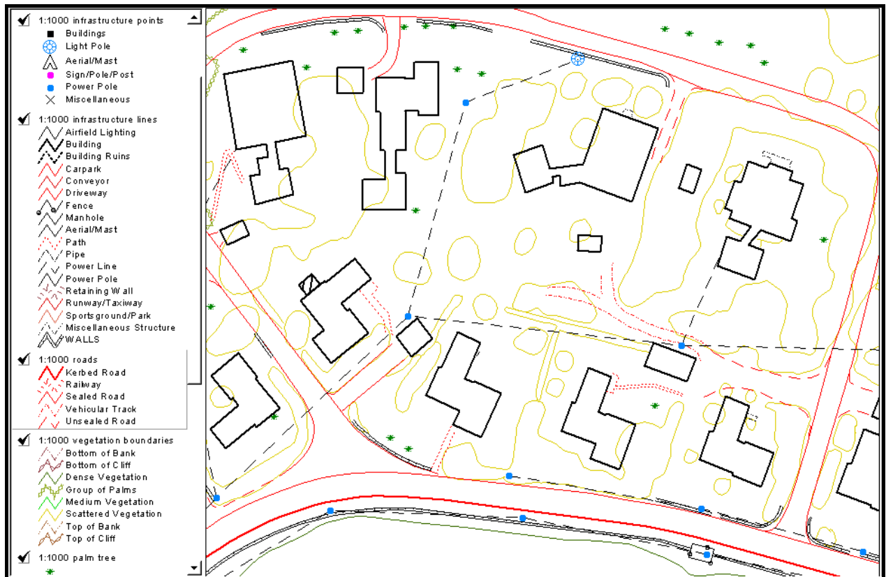
Figure 53: Screen capture of part of Rocky Point showing typical line and point features of the 1:1000 detail survey data. This data was digitised directly from the 1987 aerial photography so when compared to the orthophotography it matches very well.
