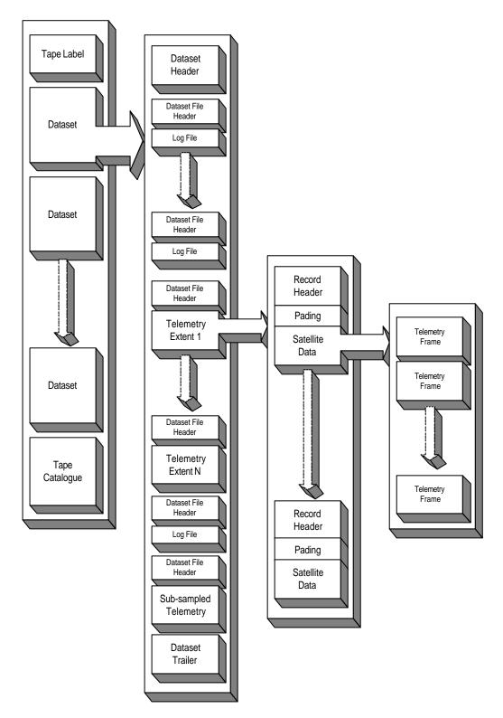
Figure 1 Tape Format Block Diagram
