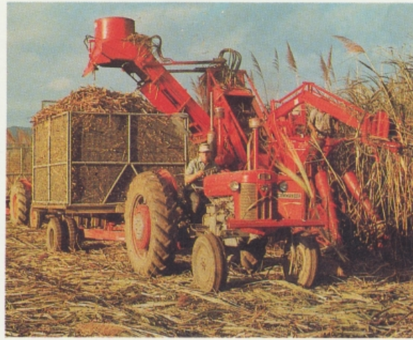
Figure 23. Cutting sugar cane in Queensland. The harvester removes the unwanted upper stalks, cuts and chops the useable cane and loads a field bin hauled by an accompanying tractor.
