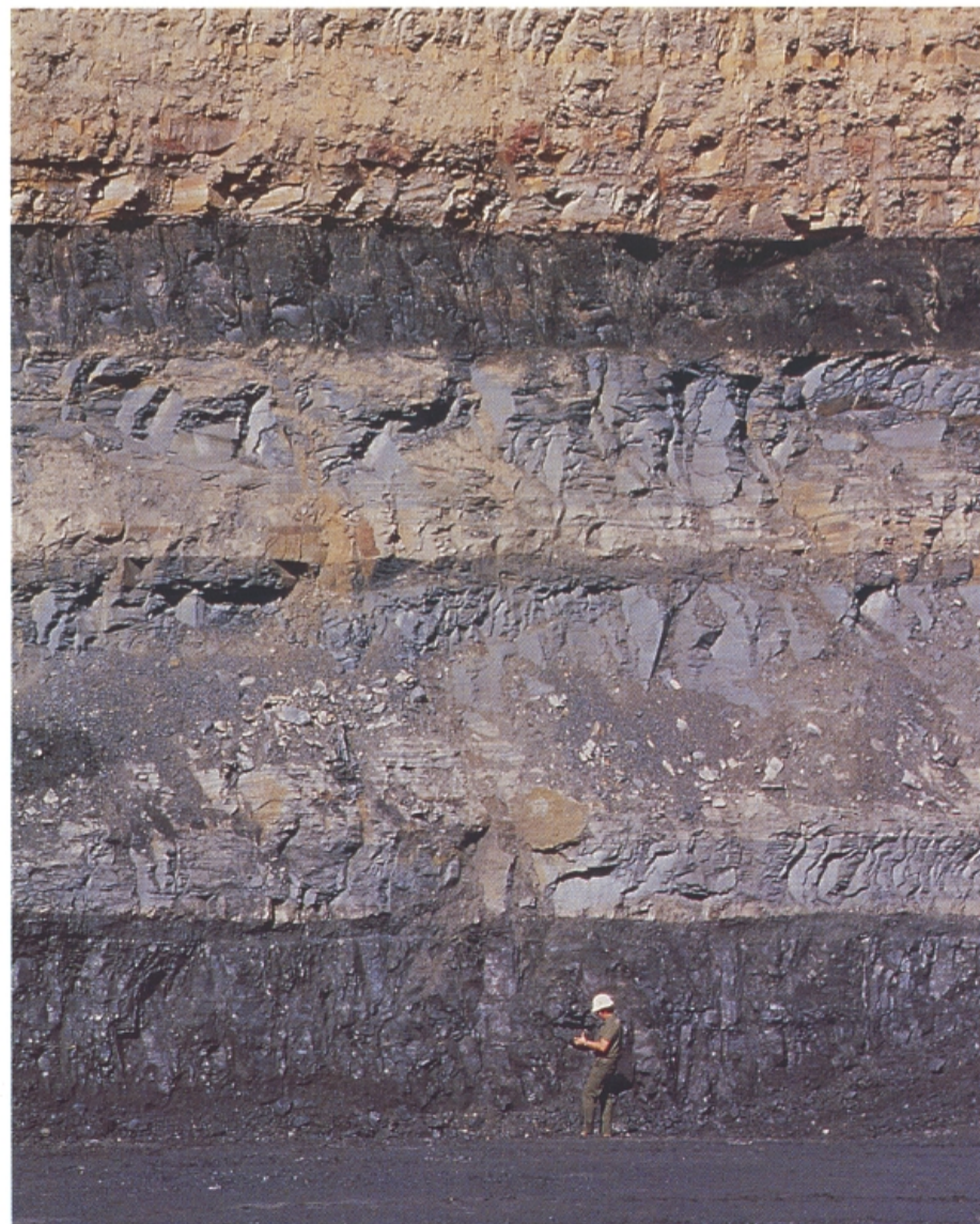
Greta Coal Measures, Drayton opencut coal mine near Muswellbrook (N.S.W.) Formed in swamps on a floodplain in the Permian, these black coal seams are interbedded with shale and siltstone and capped with sandstone.
