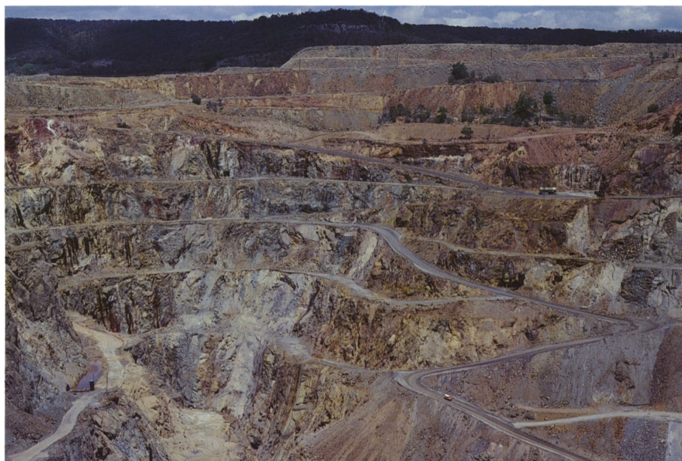
Remnant orebody in the now worked out Mount Morgan copper-gold mine (Qld) . Since its discovery in 1882 this rich Middle Proterozoic orebody, situated in a belt of volcanic rocks, has produced over 250 t of gold—an Australian record. In 1981 the orebody was exhausted but retreatment of tailings in recent years has netted around 1.5 t of gold annually. The enormous crater, quarried from a hill and now partly filled with water, is 2.5 km long, 2 km wide and 360 m deep.
