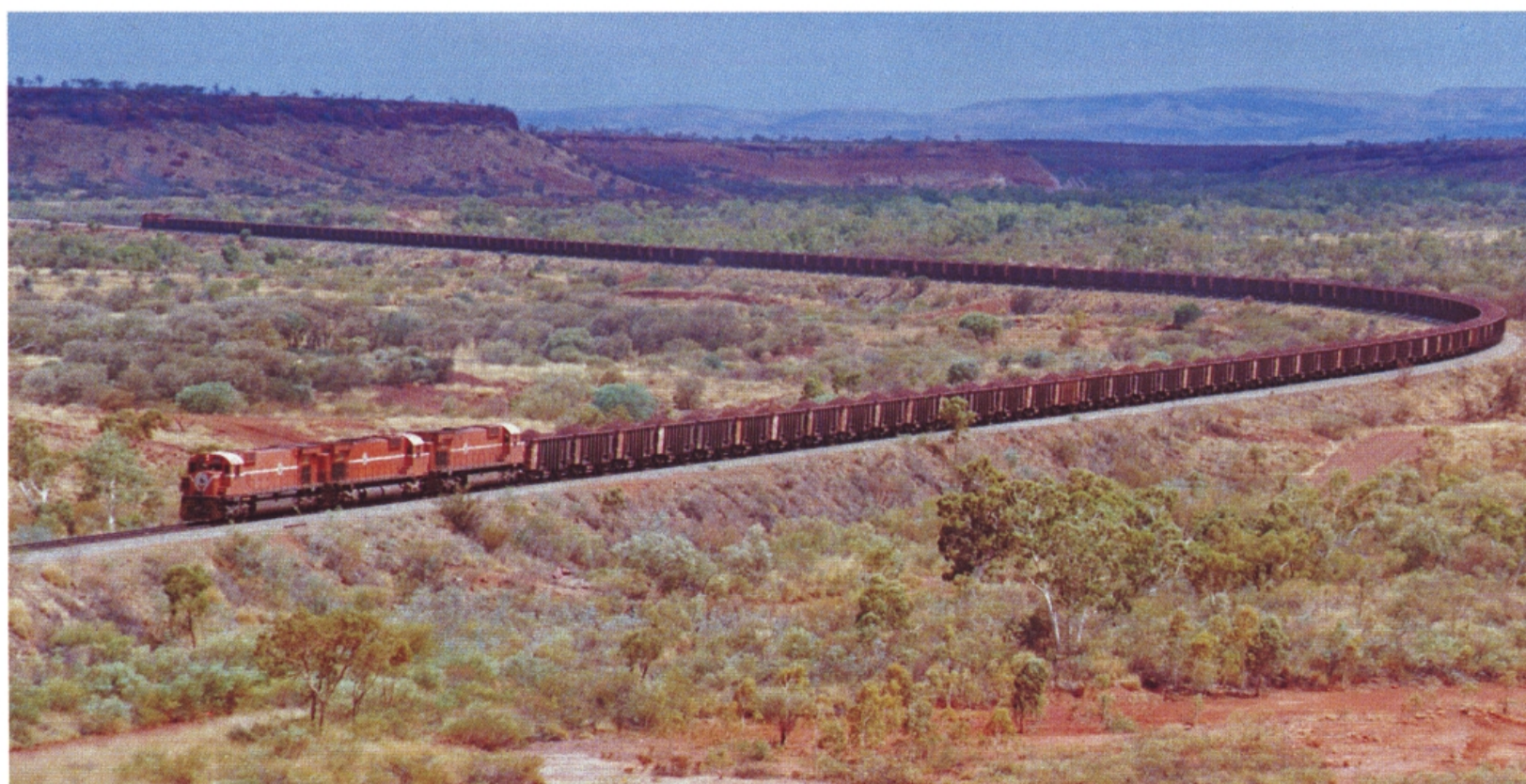
One of six daily ore trains on its 425 km journey from Newman to Port Hedland (W.A.) Around 20 trains, each carrying up to 21 000 t of iron ore in 210 wagons, travel between the Pilbara region mines and ports each day.
