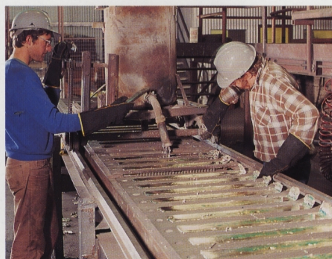
Pouring molten tin at Greenbushes (W.A.) In 1986 over 500 t of antimonial tin metal were produced at Greenbushes .
