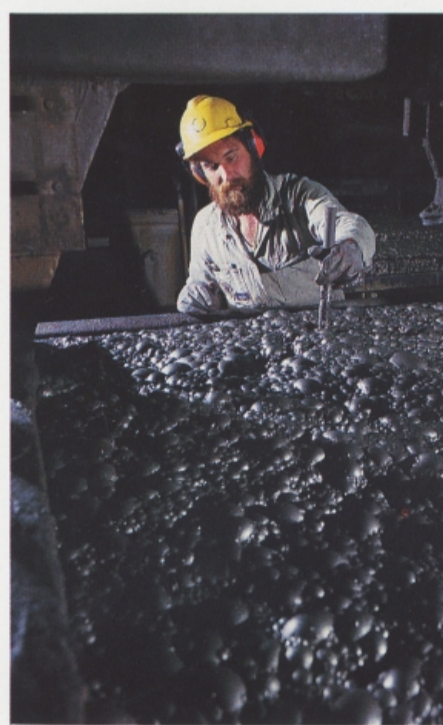
Testing the depth of froth in a nickel flotation cell at the Kambalda nickel concentrator (W.A.)
