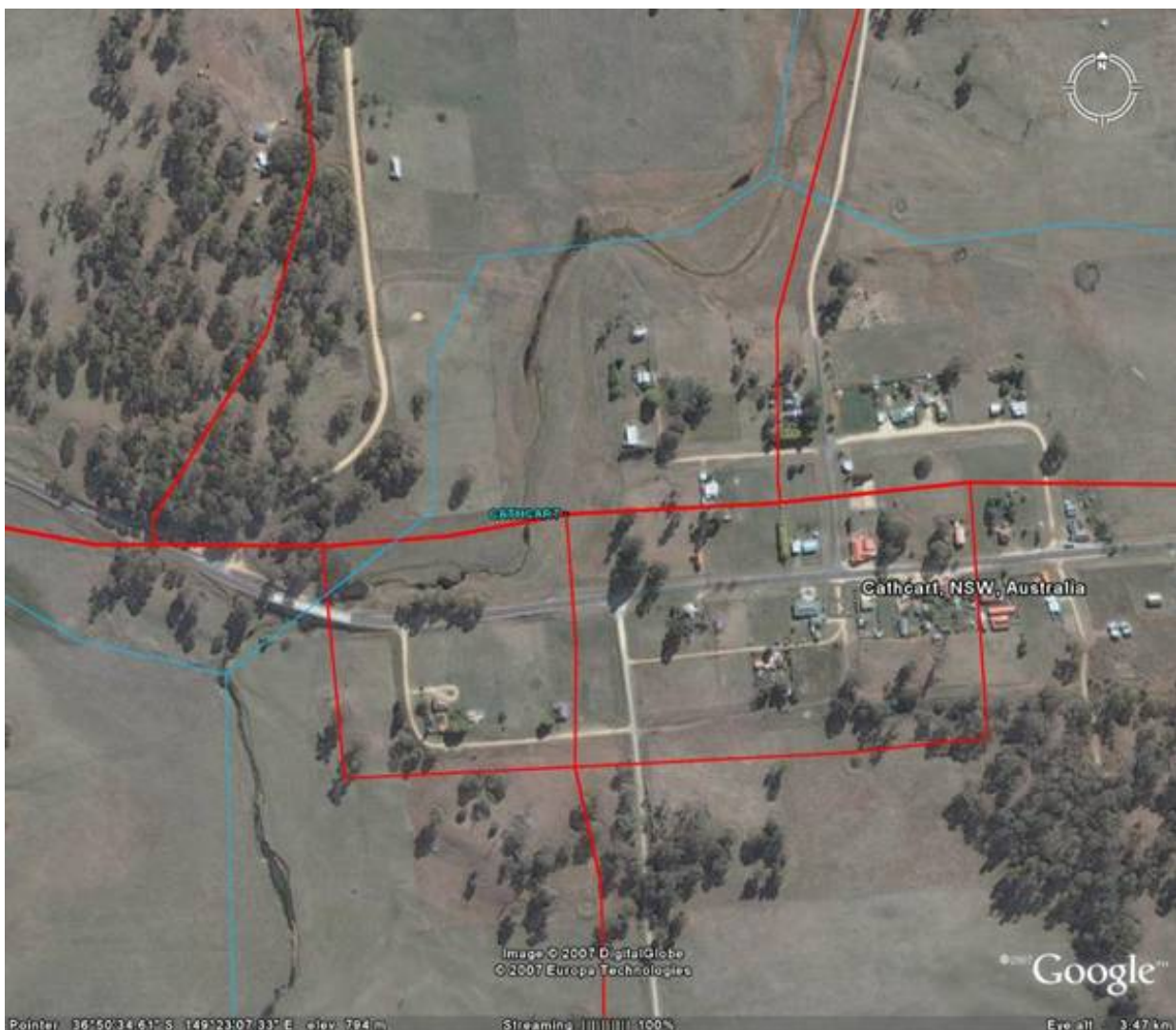
Example of spatial mismatch of features due to zoom in excess of appropriate scale
