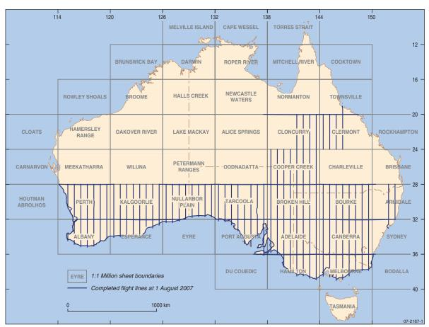
Figure 3. Flight-line pattern for the AWAGS2 magnetic and radiometrics survey showing progress to 1 August 2007.
