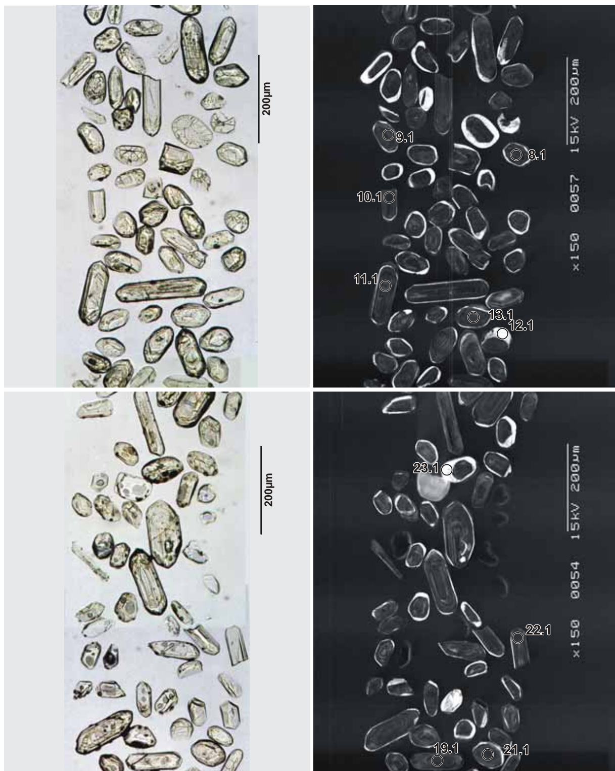
Figure 54. Representative images (transmitted light on left, cathodoluminescence on right) for sample 2002967002: biotite quartzofeldspathic gneiss, Moon Rock. SHRIMP analysis spots are labelled.
