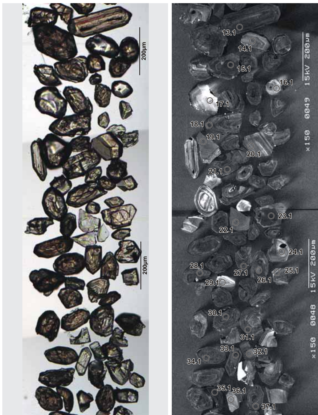
Figure 77. Representative images (transmitted light on left, cathodoluminescence on right) for sample 2004967366: meta-sandstone, Long Wong prospect. SHRIMP analysis spots are labelled.
