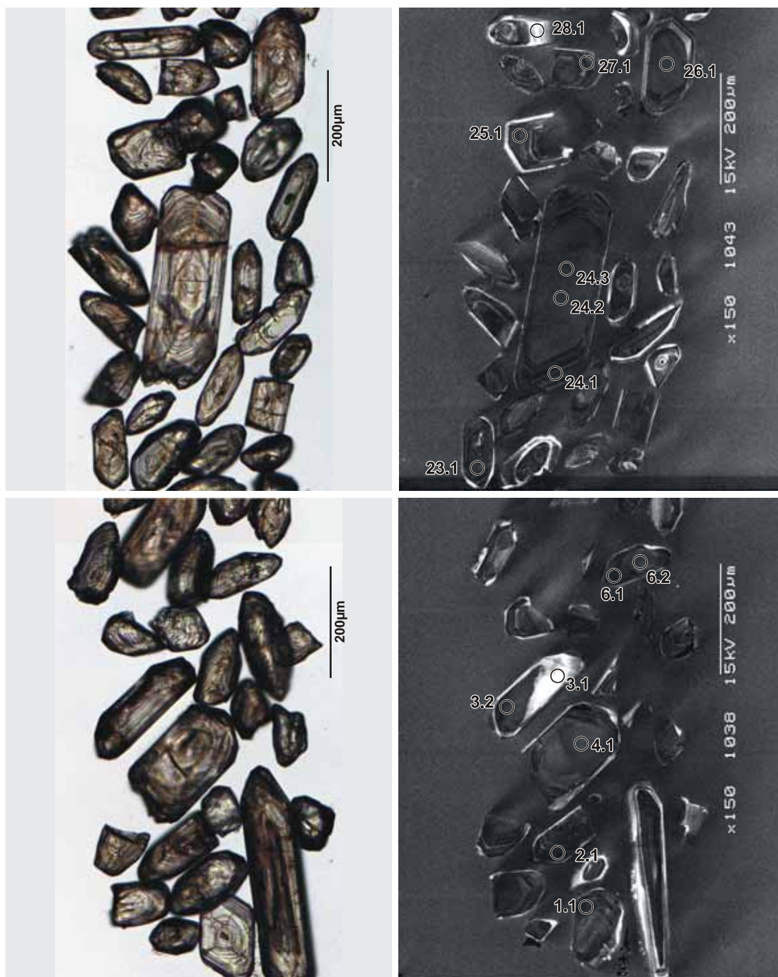
Figure 86. Representative images (transmitted light on left, cathodoluminescence on right) for sample 2004967369: porphyritic micro-diorite sill, Three-in-Hand prospect. SHRIMP analysis spots are labelled.
