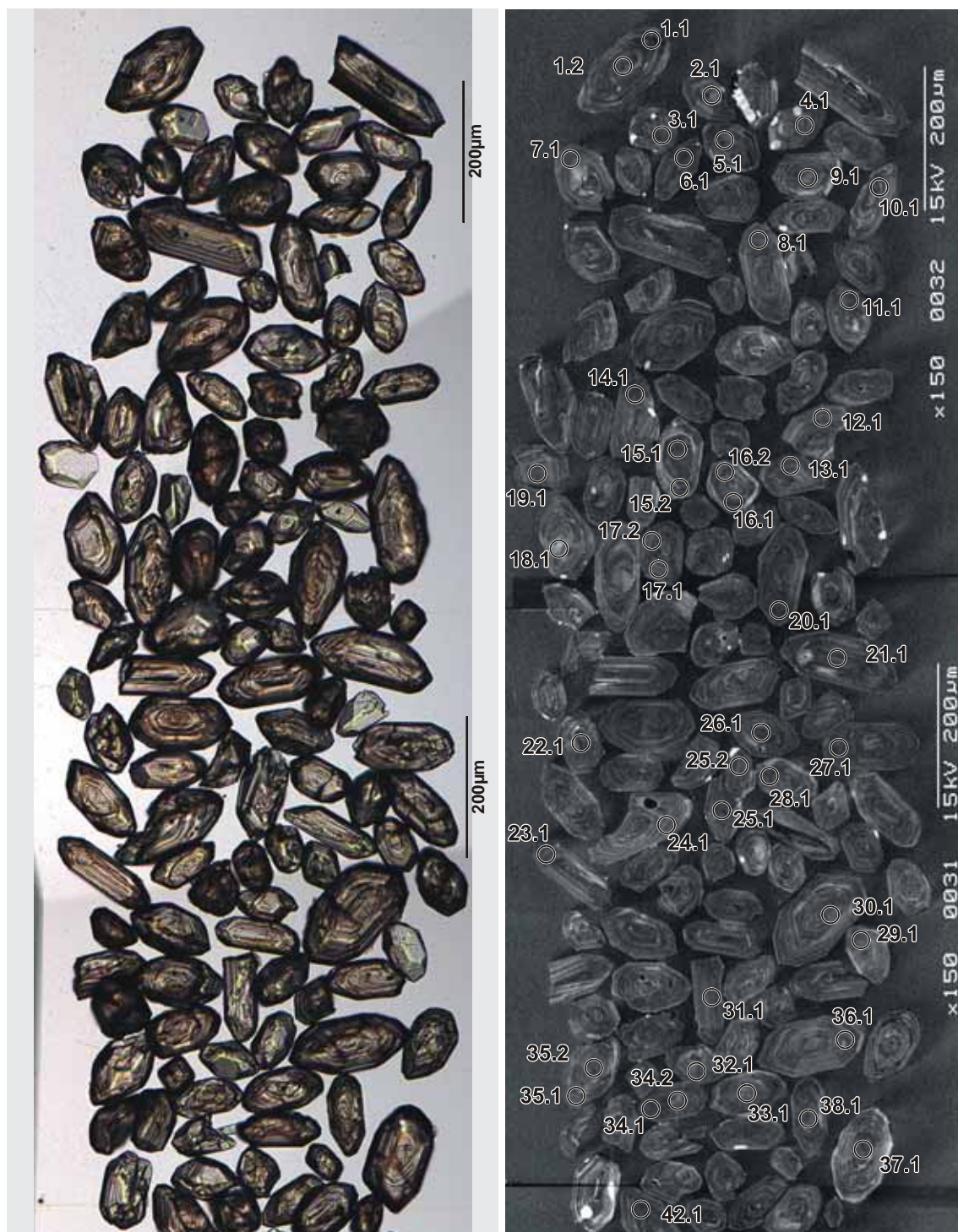
Figure 81. Representative images (transmitted light on left, cathodoluminescence on right) for sample 2004967367: volcanic meta-sandstone, Three-in-Hand prospect. SHRIMP analysis spots are labelled.
