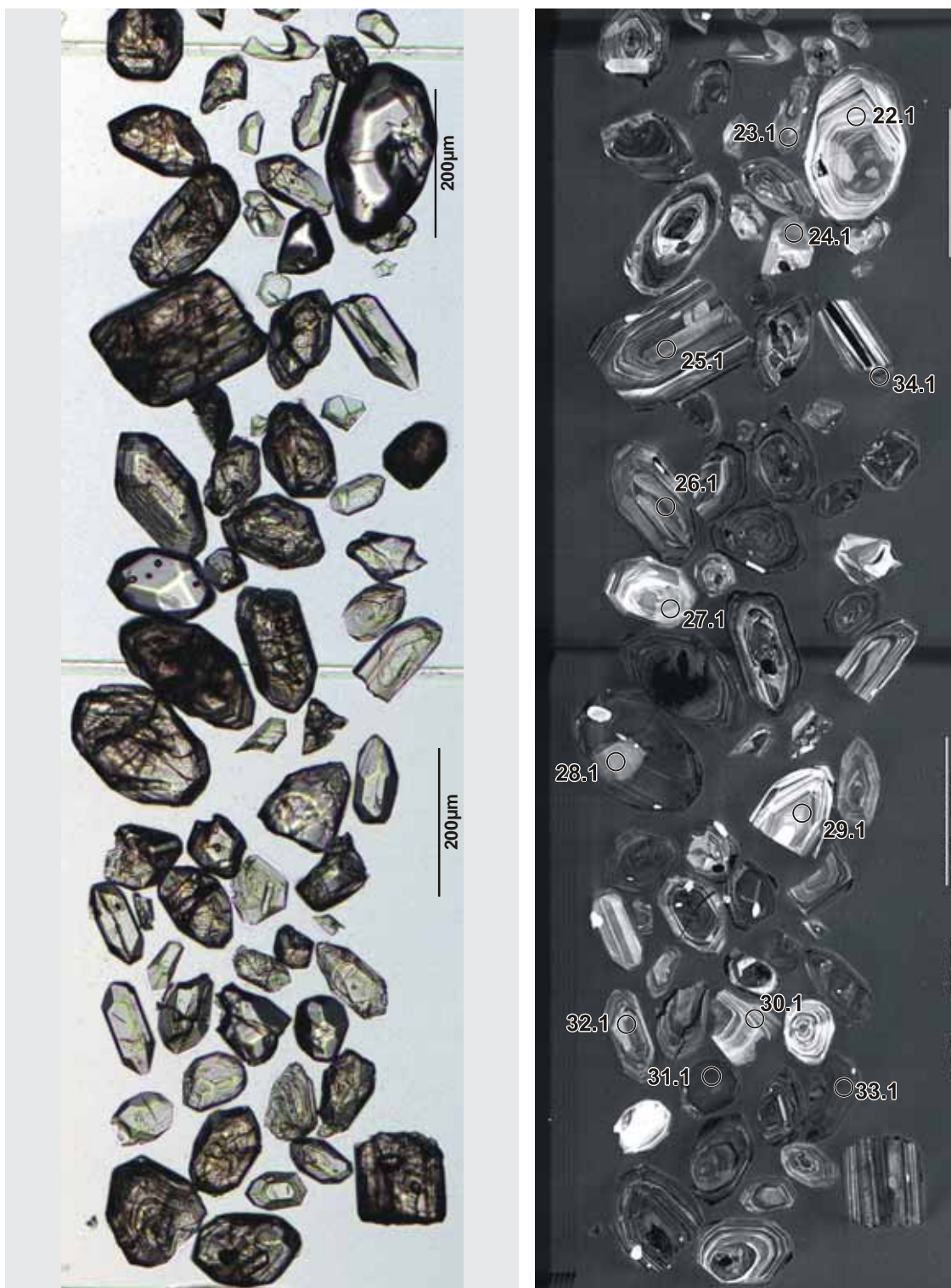
Figure 62. Representative images (transmitted light on left, cathodoluminescence on right) for sample 2004967308: volcanic meta-sandstone, Kanowna Belle. SHRIMP analysis spots are labelled.
