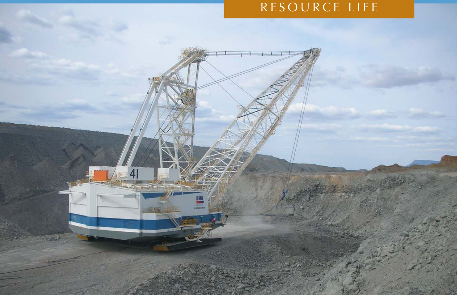
Dragline removing overburden at the Blackwater mine, Queensland (BHP Billiton Mitsubishi Alliance)
