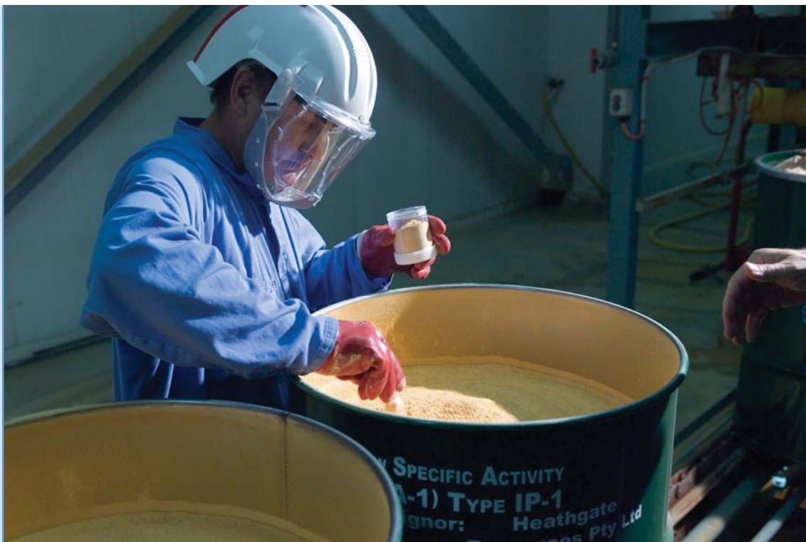
Hydrated uranium oxide ('yellowcake') in 200 litre drums ready for shipment, Beverley in-situ leach uranium operation, South Australia (Heathgate Resources Ltd)
