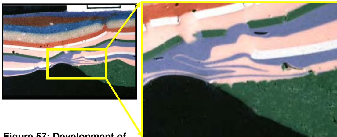
Figure 57: Development of recumbent folds in ductile lower plate (after Harris et al., 2002).
