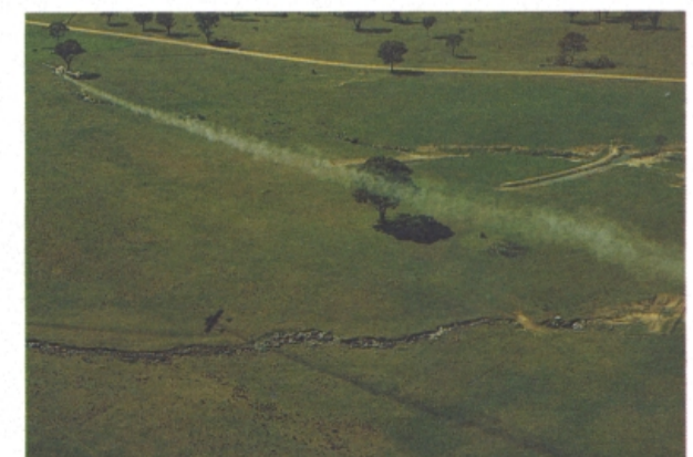
Figure 6. Aerial application of superphosphate to sown pasture on a Cd2 soil near Yass, New South Wales. The banks across the gullies are designed to prevent further erosion of the bleached, dispersible subsurface soil.
