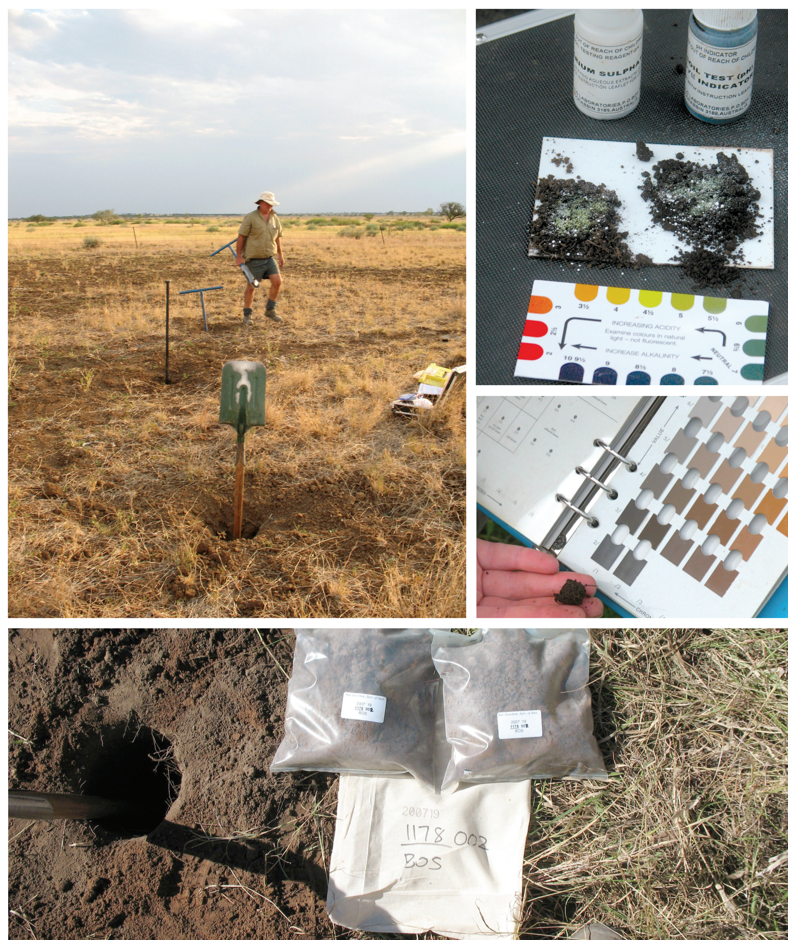
Figure 4. Auger holes, field pH, soil colour and sample bags.
