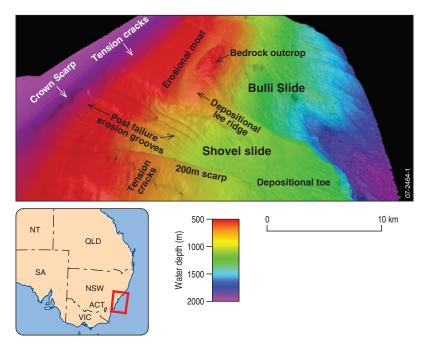
**Figure 1.** The slope failure architecture and slip-plane geometry of the Shovel Slide. Inset: the survey area off the New South Wales coast.
